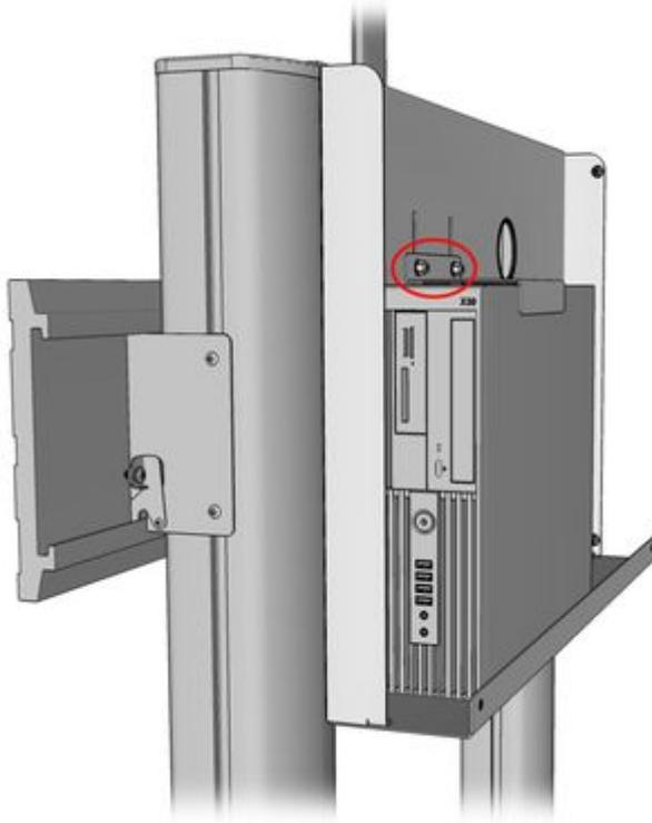
7. If the customer order includes an Interactive Input Controller (does not come standard), install by fitting the tray into the right side of the cabinet so that two of the mounting holes go over the threaded posts on the side of the cabinet.
