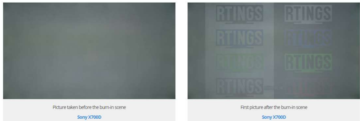
Figure 7: Example of Image Retention in an LCD (Source: Rtings)
